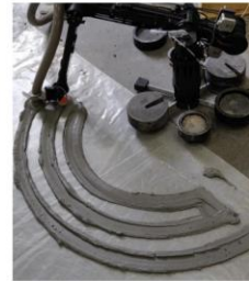
Figure 7: Process to material compatibility check showing a complete single layer curved trajectory
